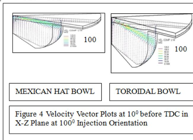
Figure 4 Velocity Vector Plots at 10° before TDC in X-Z Plane at 100° Injection Orientation
