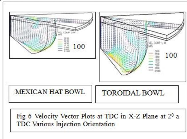
Fig 6.shows the velocity vector plots for the crank angle  $2^{\circ}$  after TDC during the expansion stroke, the piston starts moving towards the bottom dead centre.
