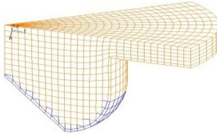
**Fig:1** Computational Sector mesh used in the engine simulation at TDC
