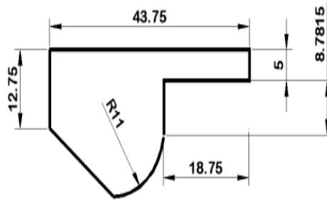
**Fig: 2.** Geometric dimensions of Piston Bowl
