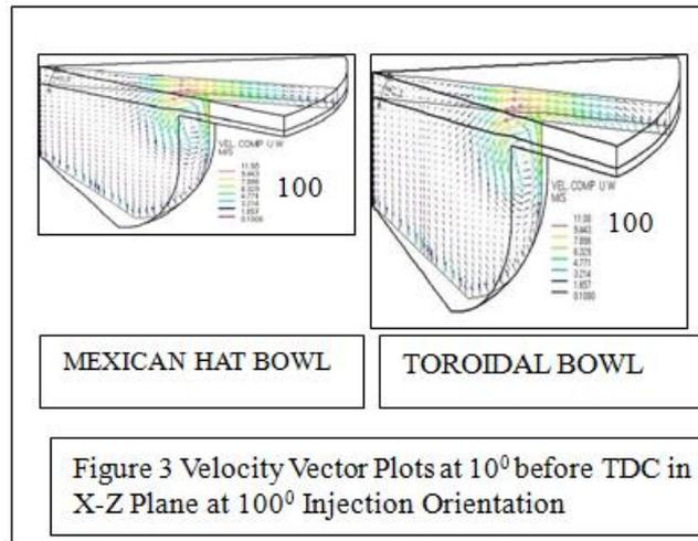
Figure 3 Velocity Vector Plots at 10° before TDC in X-Z Plane at 100° Injection Orientation
